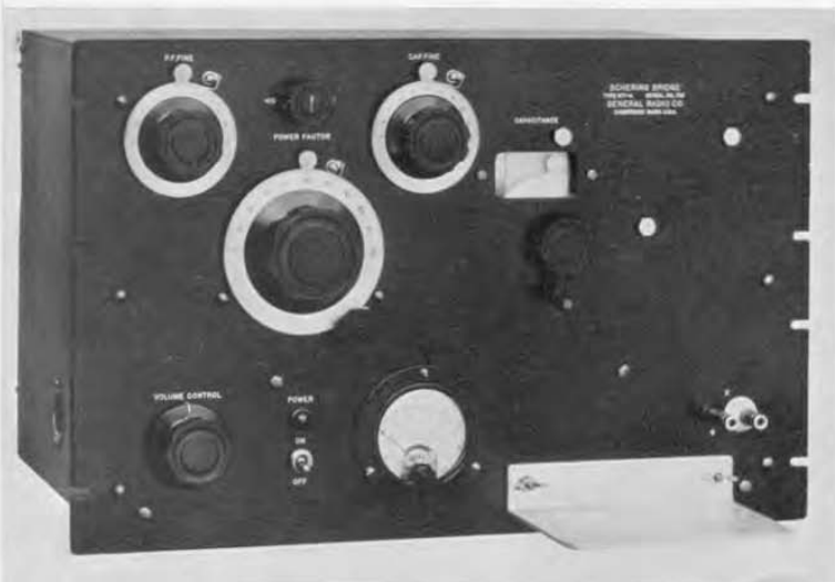
FIGURE 1. Panel view of the 60-cycle Schering bridge. Note the convenient shelf for test specimens.
